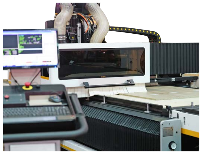
Control panel with Syntec controller; Second display for manual panel labeling
