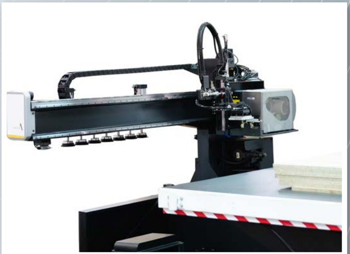
Auto Labeling System: It allows the operator to run the machine while the printer is labeling on the panel without stopping.
